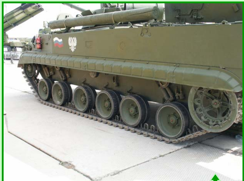
Train de roulement composé de six roues de route et trois galets supports. The suspension either side consists of six dual rubber-tired roadwheels with three track-return rollers.
